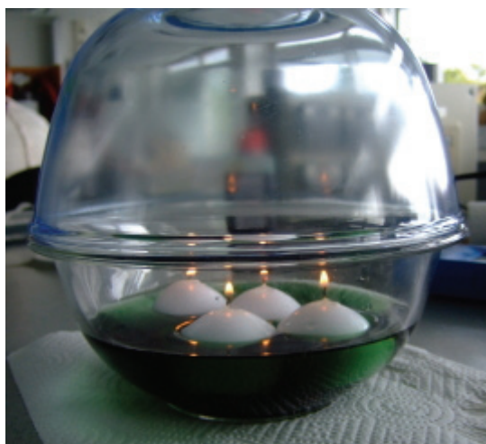
Figure 3. The bowl is covered with the other bowl. After some minutes, the candles are extinguished after they have used up all the oxygen inside. Control is the same set-up with candles unlighted.
