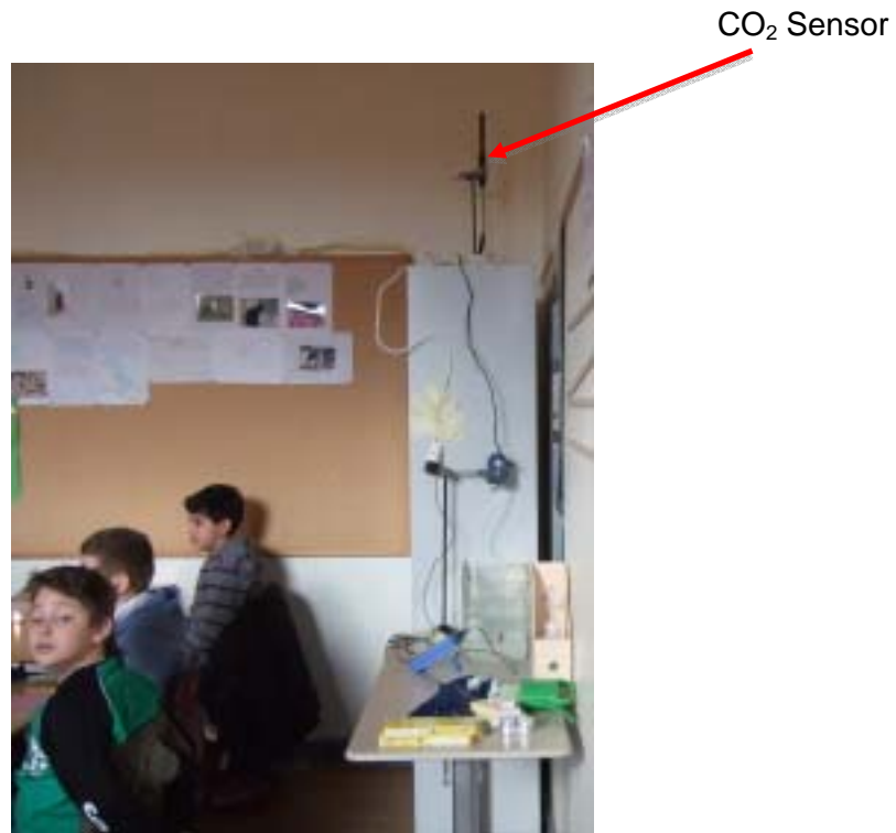
Fig. 1 Set-up. The CO 2 sensor is mounted on a stand and held with a clamp. It is placed in the back of the room on top of a shelf so the pupils will not be distracted. Free air circulation around the sensor should be ensured.
