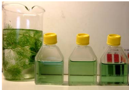
Fig 2. Fill the bottles with distilled water and add 10 drops of Mc Crumb indicator solution
