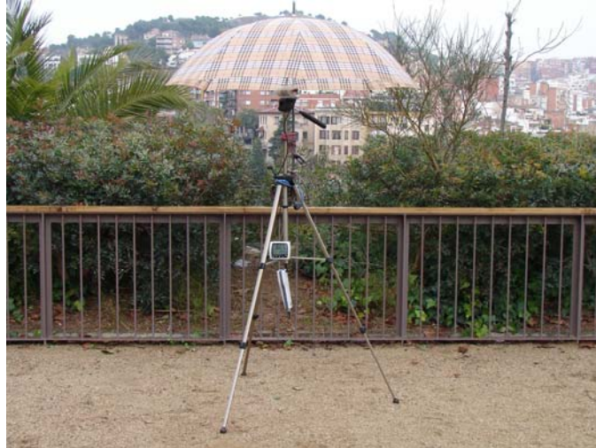
Figure 1. Experimental set up for taking CO 2 measurements along a transect
