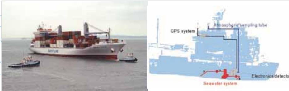
In order to continuously obtain new data, commercial ships such as the MV Benguela Stream (cargo ship to the left) were equipped with a CO<sub>2</sub> measurement system. With the help of these continuous data, scientists can monitor the North Atlantic sink and quantify how the CO<sub>2</sub> uptake changes over time and varies for different latitudes. (Source: T. Steinhoff and U. Schuster).
