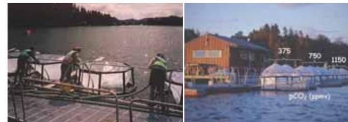
How does the marine ecosystem react to a doubling of today's atmospheric CO<sub>2</sub> concentration? In Norway, near Bergen, large plastic bags (called „mesocosms“, which literally means „medium worlds“) with artificially CO<sub>2</sub>-enriched water enable the consequences of this enrichment on marine life to be observed „in situ“. (A. Volbers, U. Riebesell)
