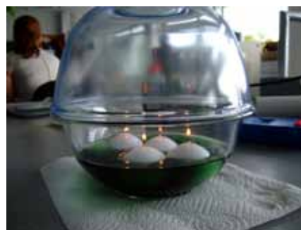
The bowl is covered with the other bowl. After some minutes, the candles are extinguished after they have used up all the oxygen inside. The control is the same set-up with candles unlighted.
